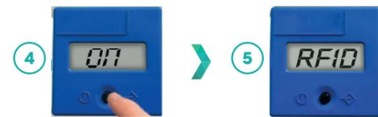
4. Turn-on the rapiread» by pressing the black button. Reader runs a self-test, during the self-test «wait» is displayed. after an audible beep signal, «on» is displayed. To perform a reading, press the black button again once for 1 second..
