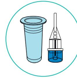
1. UniSampler™ Device contains Collection Tube (1) and Blood Collector with Cap (1)
