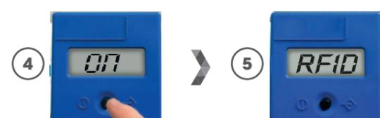
4. Turn-on the RapiRead™ by pressing the black button. Reader runs a self-test, during the self-test «WAIT» is displayed. After an audible beep signal, «ON» is displayed. Keep pressing black button till display shows RFID.
